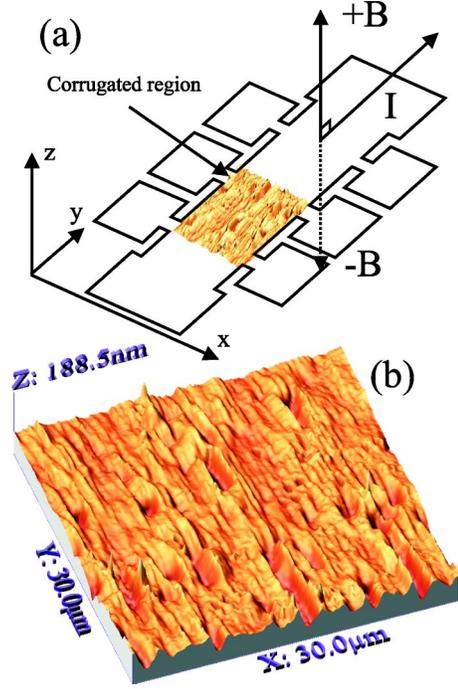
FIG. 1. (a) Scheme of the sample hall bar showing the location of the corrugated region. (b) Atomic-force microscope image of a small region ( $900 \mu\text{m}^2$ ) of the corrugated region of the sample.
