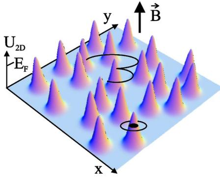
FIG. 4. Scheme of an array of two-dimensional antidots, formed by electrostatic Gaussian potentials distributed randomly.  $E_F$  represents the Fermi energy and  $\vec{B}$  the magnetic field vector.
