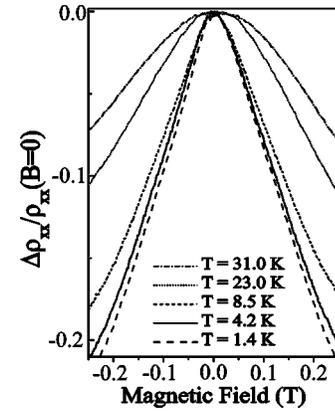
FIG. 3. Negative magnetoresistance at low magnetic field, for different temperatures between 1.4 and 31 K.
